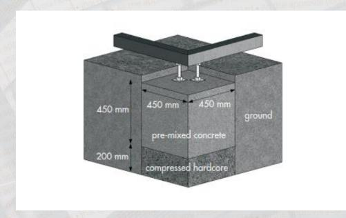
Part A (Structure) of the building regulations gives further guidance for the design of foundations, however it is acknowledged that this is based upon the
